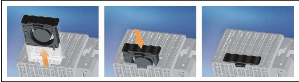
Figure 11: X20 CPUs - tool-free fan replacement
